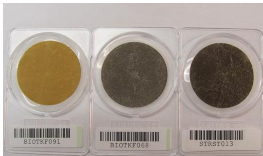
Figure 3. Pictures of Teflon filter samples of biomass smoldering, biomass flaming, and diesel exhaust emissions, as described in Figure 2.
